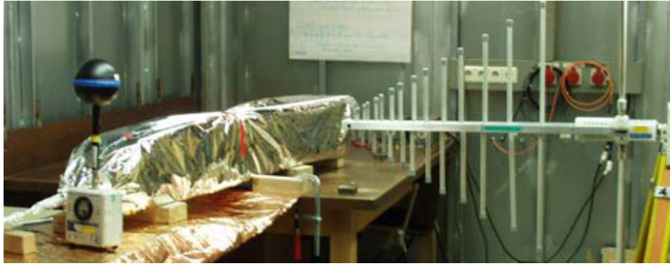
Figure 2.42: The picture was taken during the EMI test of a TRD prototype at the MPE in Garching. From left to right one can see the electric field sensor (black globe), the TRD prototype (wrapped in MLI) and the antenna of the emitter. [S. Schael, AMS02 TIM April 2003]
