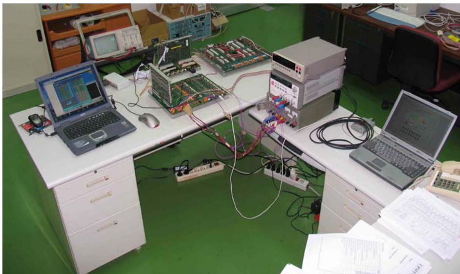
Figure 2.51: The UPSFEv2 test setup, as it was used during the quality control of the QM2 production at CSIST in Taiwan. The setup from left to right: The laptop computer was used to control the UPSFEv2 via an EPPCAN box and an USCM. The oscilloscope is needed for the measurement of the timing of the solid-state fuses and the linear regulators. Next is the UPSFEv2 itself, sitting in the UPSFEv2 test backplane. On its right are two power supplies, one for the digital part, one for the analog part together with the digital multi-meter used for monitoring the currents. The computer used to control the DMM and to log the data from it is located right next to it.
