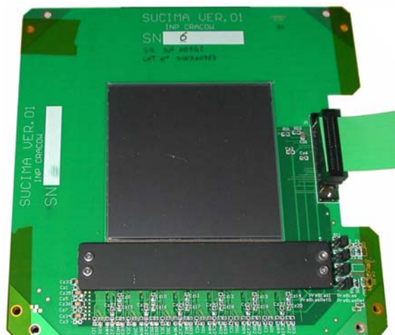
Figure 4.7: A picture of the silicon micro-strip detector of SUCIMA mounted on its hybrid.
