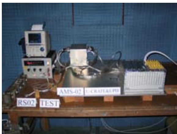
Figure 5.68: Experimental arrangement of the QM2 EMI test in Taiwan.
