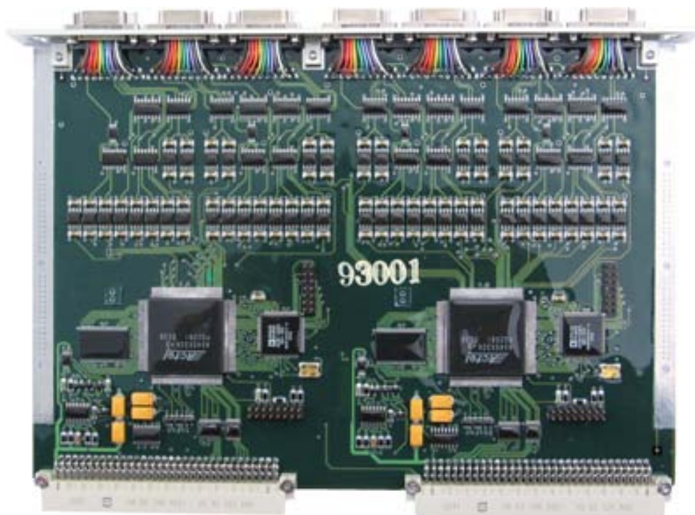
Figure 5.22: Front side of the UDR2 board. Two CDPs feature two-fold redundancy.
