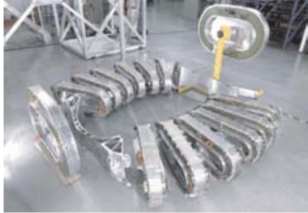
Figure 2.7: Picture of the AMS-02 coils: left and right are the dipole coils, in between are the racetrack coils for the flux return.
