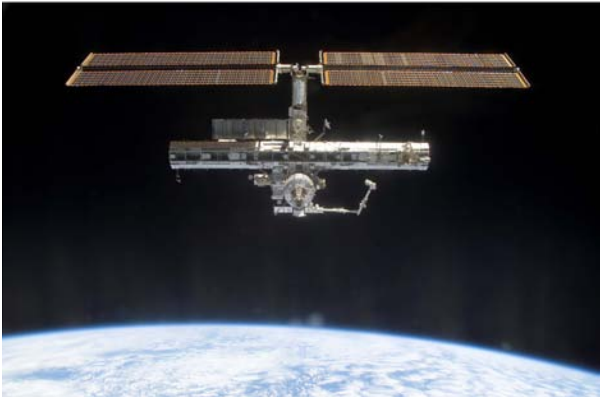
Figure 3.3: Full view of the International Space Station. Photographed on December 2nd, 2002 by a crew member on board the Space Shuttle Endeavour following the undocking. The newly installed Port One (P1) truss now complements the Starboard One (S1) truss in center frame.
