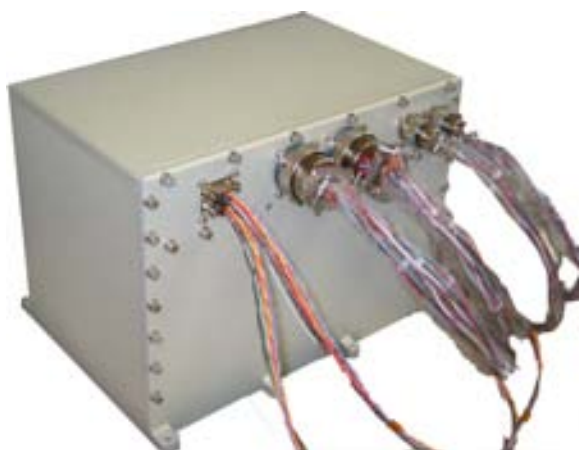
Figure 5.41: Assembled Power Distribution Box for the TRD (UPD-Box). Mil-Spec connectors coupled the supply lines to the UPD-Box. 15-pin micro-d pigtail connectors guide the slow control communication from the UBPv2 to the UPD-Box.
