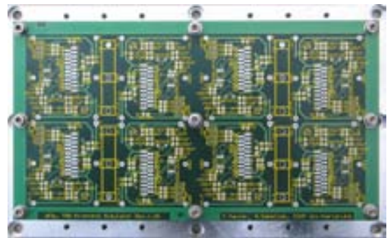
Figure 5.80: UFS PCB, mounted on support mechanics.
