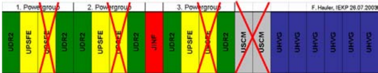
Figure 5.50: Changes of module arrangement on UBP due to weight reduction.
