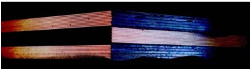
Figure 2.42: Photo of the assembly of three ECAL layers. In adjacent layers the pointing direction of the fibers change by 90^\circ to obtain the three-dimensional imaging capability.
