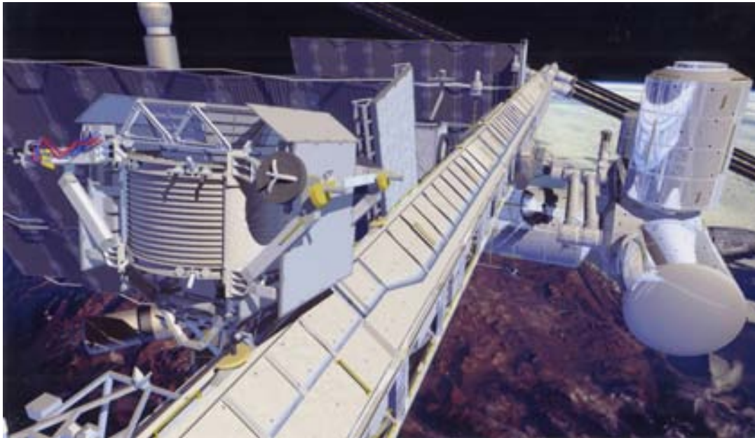
Figure 1.1: Drawing of the AMS-02 detector mounted on the International Space Station. Source: Lockheed Martin.
