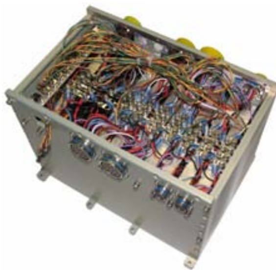
Figure 5.42: Inner view of the UPD-Box assembly test. The length of the cables will be reduced to a minimum in the final QM2 assembly.
