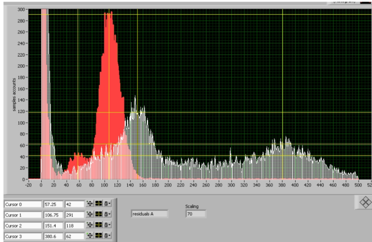
Figure 6.6: Energy spectrums of ^{55}\text{Fe} and ^{109}\text{Cd} sources taken from the BOT electrode at a gain of 5000 using the DP-GP5 readout electronics. The energy resolution is 42% FWHM at 5.9keV.
