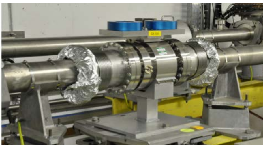
Figure 16: a picture of a new stripline BPM on the LINAC2 to PSB beam-line
