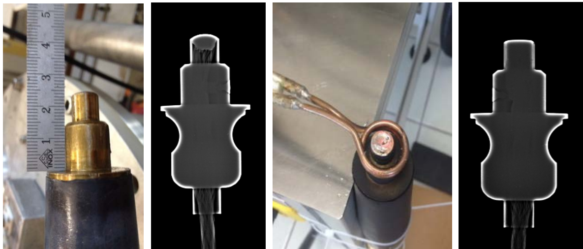
Figure 7: Improvements of the LHC HV connectors; from left to right: a view of the connector, the x-ray of the connector before intervention showing voids in the weld, the induction welding coil, the x-ray of the repaired connector.
