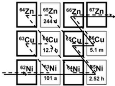
Fig. 1: The s-process reaction path in the Ni-Cu-Zn region during He core burning (dashed lines) and the C shell burning (solid lines) [4]
