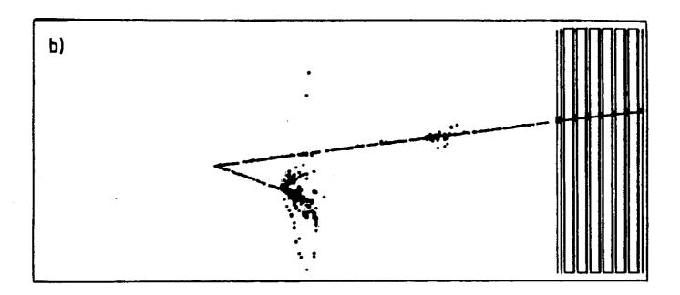
Figure 3: Example of trident production candidate event (a) and single pion production candidate event (b) in the CHARM II detector. The neutrino beam enters from the left. Each point in the calorimeter represents a hit wire. In the muon spectrometer the drift chamber hits are shown together with the reconstructed muon tracks.
