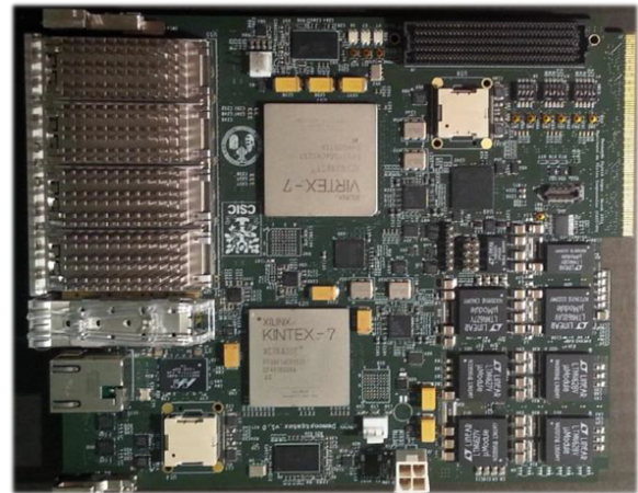
Figure 7: Upgraded Read out Driver for the back end electronics.
