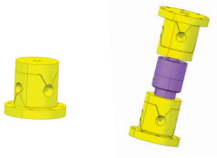
Figure 4.2: The flexural hinge designed by K. Artoos (left) and the flexural hinges combined with a PI piezo actuator (right).
