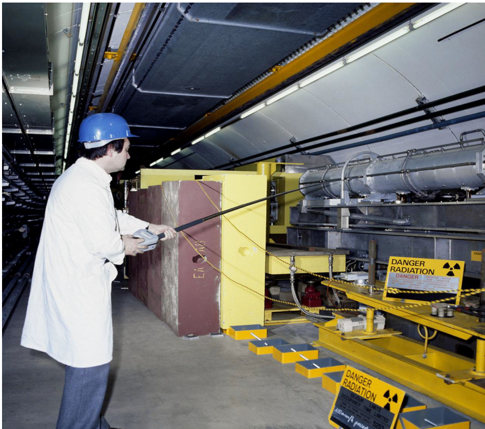
Figure B.2 – Manual measurements of radiation levels.
