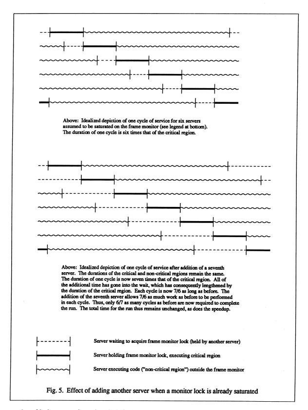
number of lock attempts for a given lock, is then subtracted from the accumulation of TSPINLOCK times for that lock, yielding the total critical-region contention time associated with the lock. Division once again by the number of lock attempts for the lock yields the average critical-region contention time per
