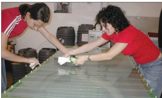
Two high-school students who are part of the Italian EEE project build an MRPC muon chamber in CERN's Building 29.
