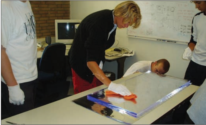
School students construct a scintillator detector for one of the five regional clusters for the HISPARC cosmic-ray detector array.
