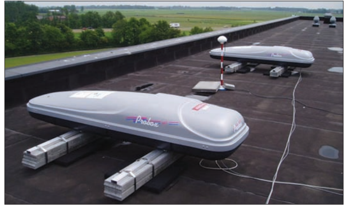
Boxes containing cosmic-ray detectors on a school rooftop as part of the HISPARC project. (Photos courtesy Ilka Tanczos.)
