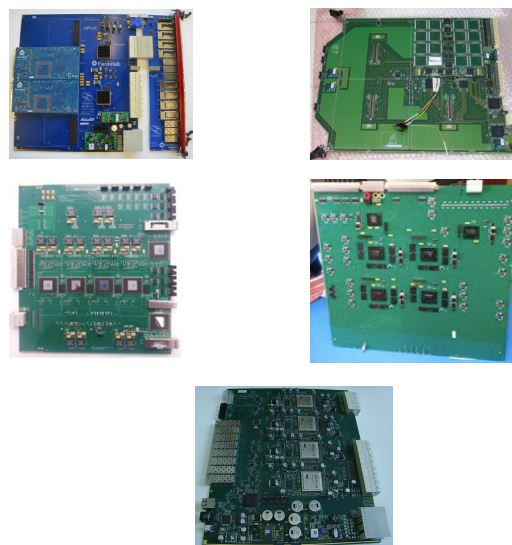
Fig. 2. The prototype of individual FTK components: DF with RTM, AMB with one LAMB mounted, AUX, SSB, FLIC.
