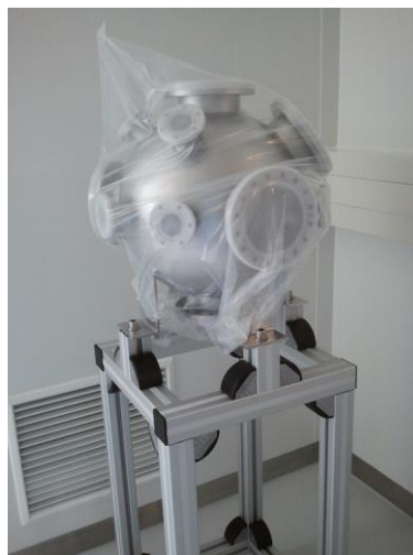
Figure 15: The sphere preparation chamber is waiting for the assembling in the clean room.
