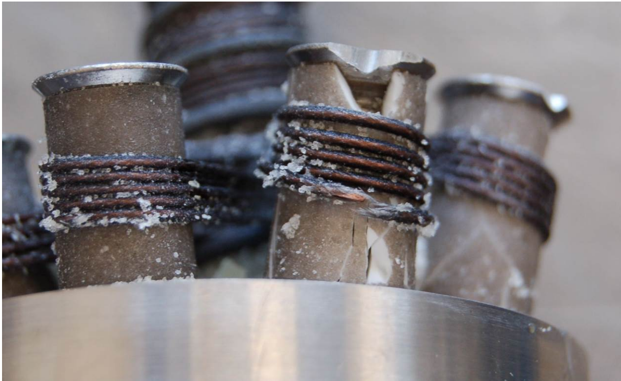
Figure38: Showing broken wire and fractured macor winding post after removal of epoxy resin
