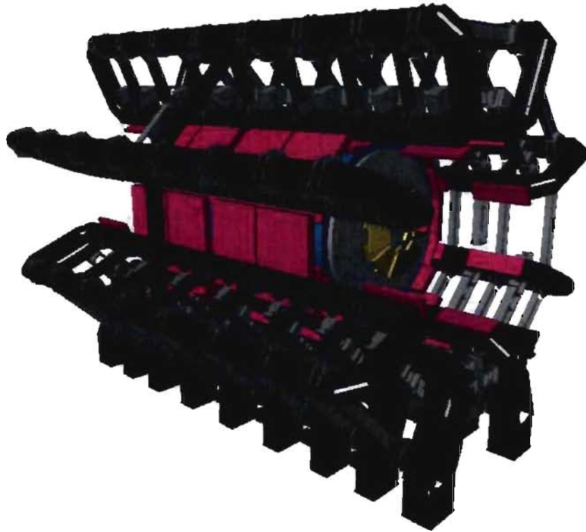
Figure 2.5: External magnet system composed of eight toroids of 26 meters length with an outer diameter of 19.5 m . It is by far the biggest magnet system ever built. The components in magenta and green are the outer section of the inner barrel containing the calorimeters and the inner detector, included in this figure just to give an idea of the size of the system.
