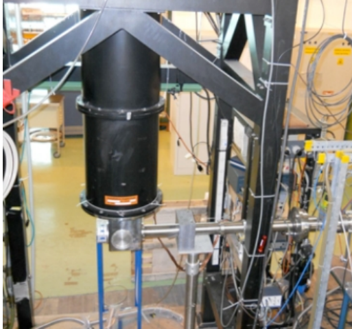
Figure 1. (Left) NICOLE setup with shown significant parts of the system, support pillars and the cryostat. (Right) VANDLE system in the 50 radius ring as implemented at HRIBF.
