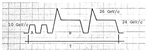
The cycle time  $\tau$  must be a multiple (integer) of the A cycle time. Today, A is  $\geq 1.2$  s and may be repeated up to five times whilst B is typically repeated three times with a cycle time of 2.4 s.
