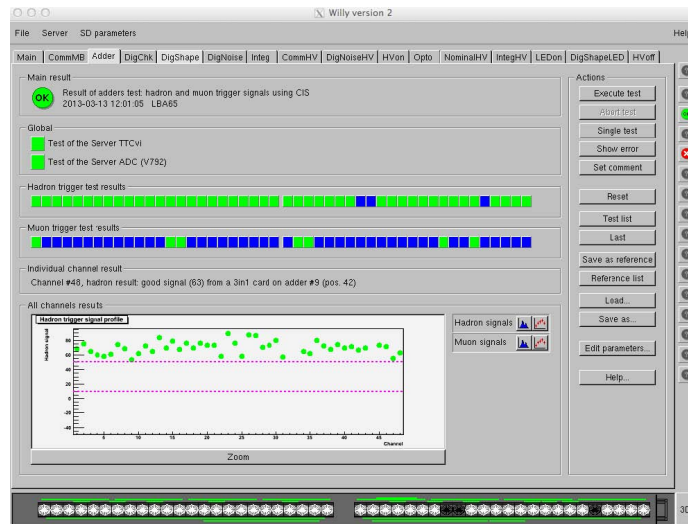
Figure 8. Picture of the Willy GUI showing the adder test.
