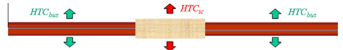
Fig. 7. Sketch of the bus bar and interconnection heat transfer coefficients: HTC_{bus} and HTC_{ic} .
