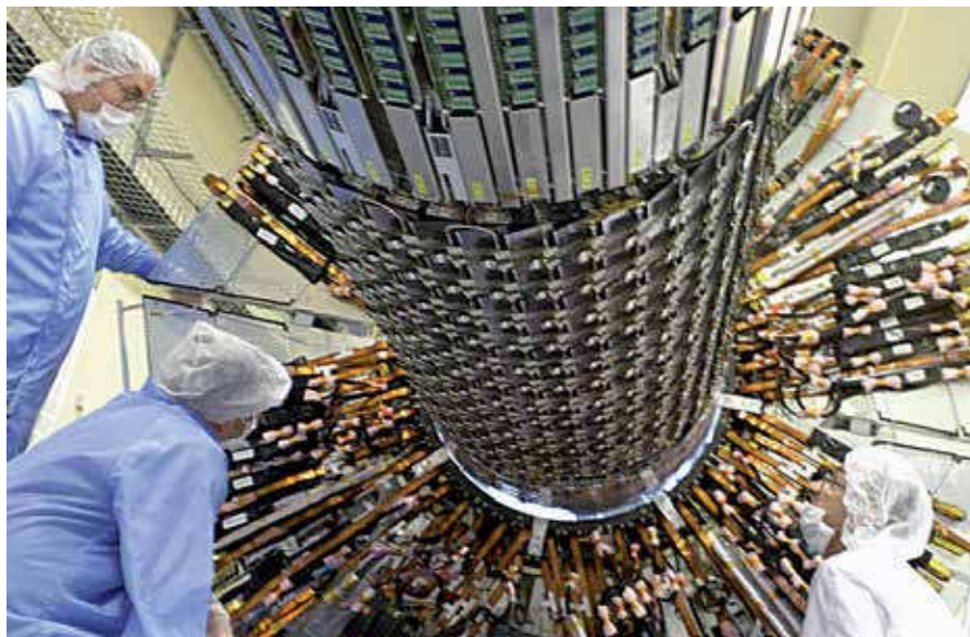
Silicon strip detector technology being readied for CERN's ATLAS experiment.
