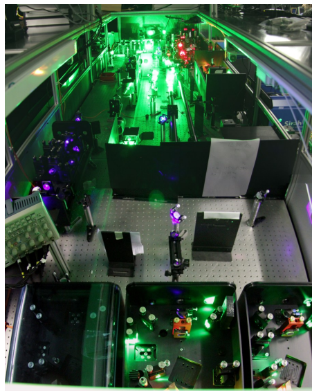
Figure 2: Panoramic view of the RILIS laser table setup (courtesy of S. Rothe). The three newly added Ti:Sa lasers are shown in the lower part of the picture. The upper part shows the focussing and launch setup commonly used by all RILIS lasers.
