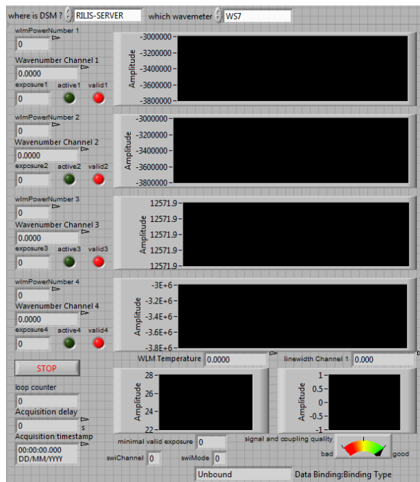
Figure 26: Wavemeter readout VI front panel. Each channel value is displayed numerically on the left and graphically on the right. Additional informational values regarding the current status are displayed by indicators on the lower part.
