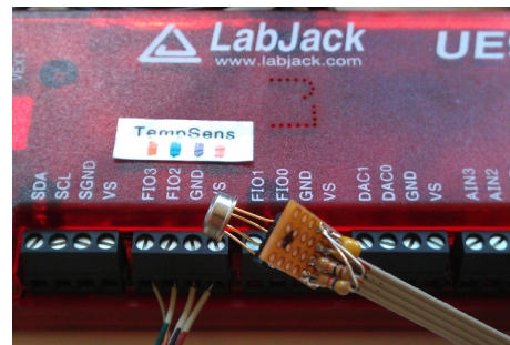
Figure 9: Temperature sensor connected to the screw terminals of the LabJack data acquisition device.
