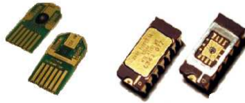
Figure 2. RadFET dosimeters from REM Ltd. (two from left) and from Tyndall National Institute (two from right)
