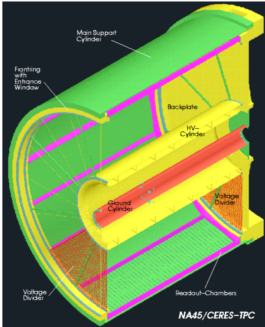
Figure 2.5: Cross section through the CERES TPC.
