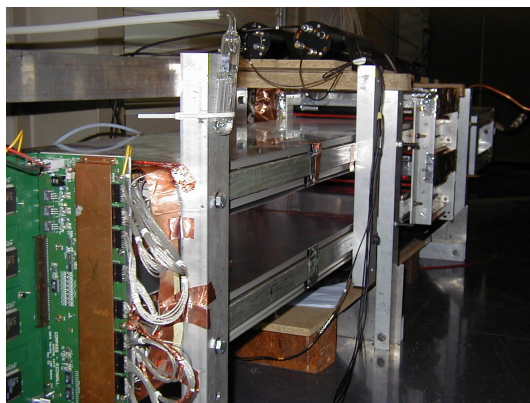
Figure 58: RW FSP with extra aluminum plates between biplanes.
