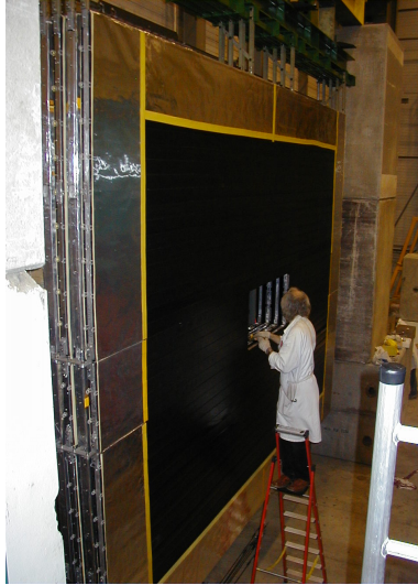
Figure 73: Rich Wall in “park” position, without FE electronics.
