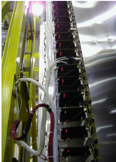
Figure 74: Rich Wall in work position, with FE electronics.
