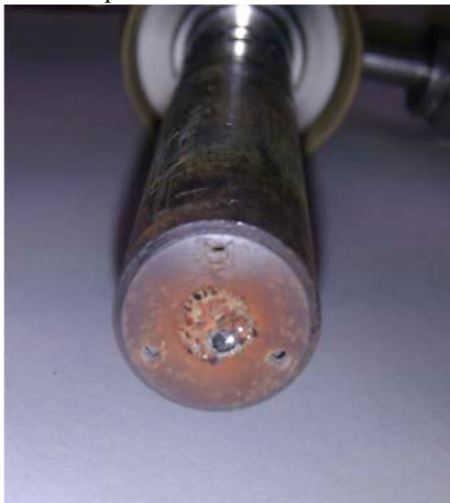
Figure 3: Oven tip clogged with lead and lead oxide.
