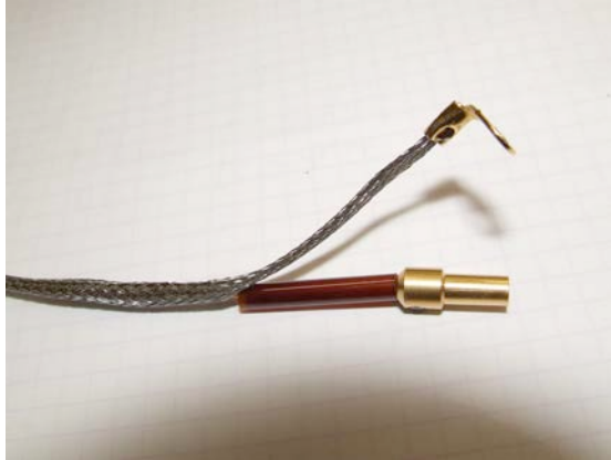
Figure 2: Modified electrical connection for the intermediate electrode.
