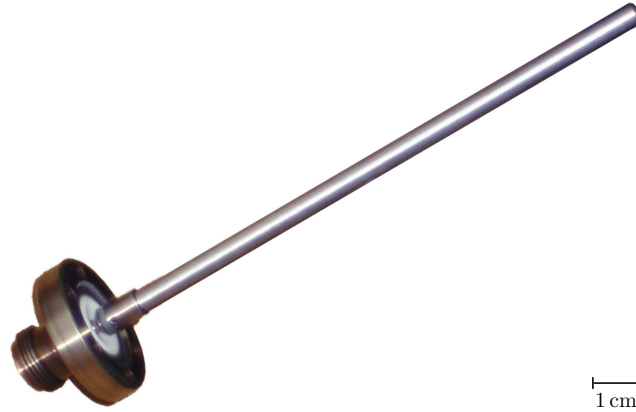
Figure 4.12: (Color) Example of a feedthrough equipped with an antenna. Four such devices are used around the cavity: Two to couple the RF power into the cavity and two to pick up the signal. This allows selective excitation of the wanted mode as well as monitoring the mode pattern inside the cavity.
