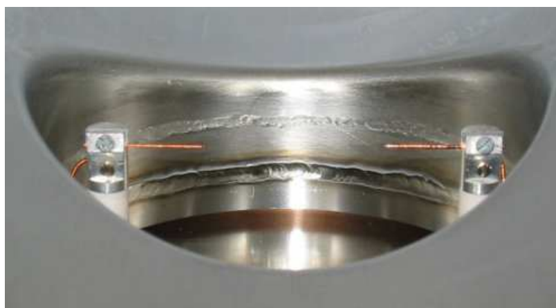
Figure 4.2: A SPS linear wire scanner in its initial parking position.
