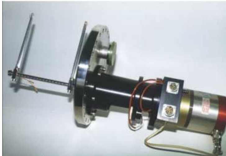
Figure 4.3: SPS rotational wire scanner mechanism.
