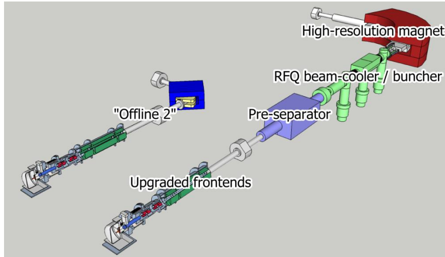
Figure 7: Layout of a Mark-II HRS offline test stand
