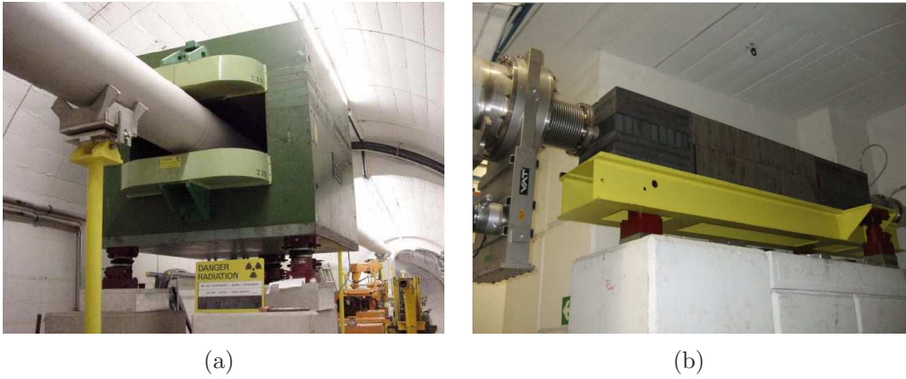
Figure 2.5: The sweeping magnet (a) and the second collimator defining the beam size (b).
