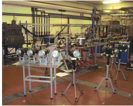
Figure 4: The ^8\text{B} experiment. 8 Photo Multiplier Tubes cover neutron angles from 15^\circ to 140^\circ in the lab frame.
