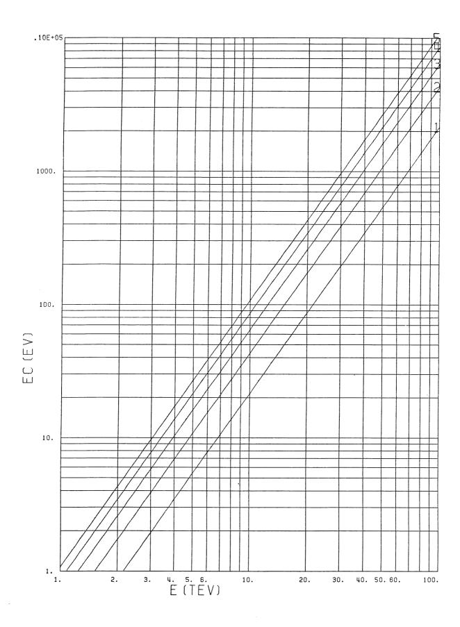
6. Critical synchrotron radiation photon energy  $E_{\rm C}$  in eV versus beam energy E in TeV. The parameter is the dipole field B, taking values 2, 4, 6, 8, 10T for curves 1, 2, 3, 4, 5 respectively.
