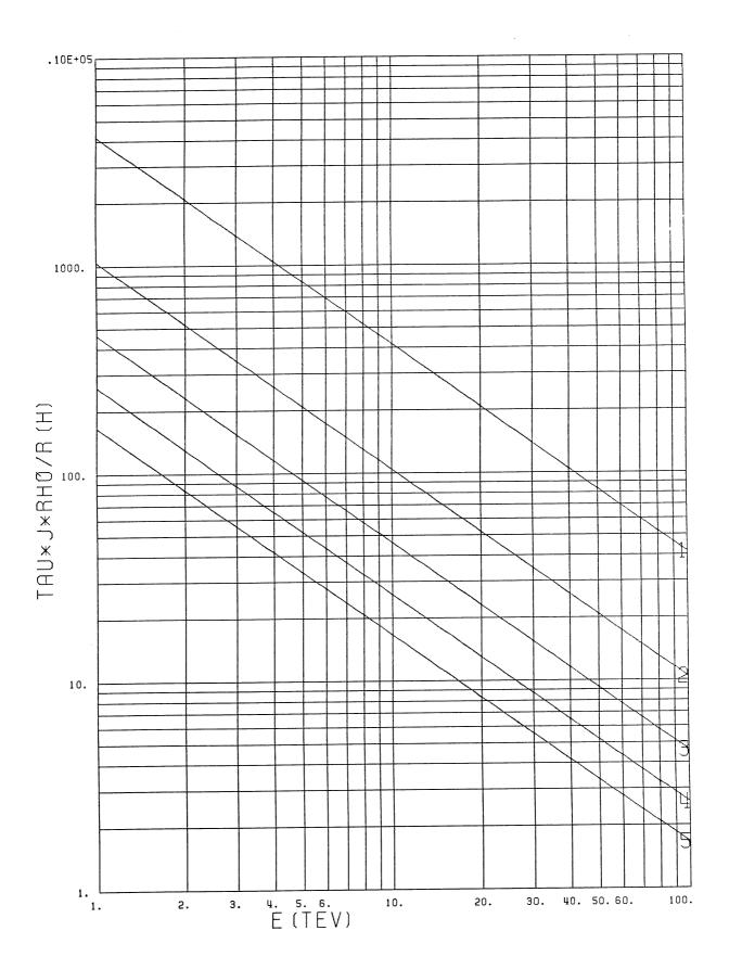
5. Product  $\tau J_P/R$  for synchrotron radiation damping in hours versus beam energy E in TeV. The parameter is the dipole field B, taking values 2, 4, 6, 8, 10T for curves 1, 2, 3, 4, 5 respectively.
