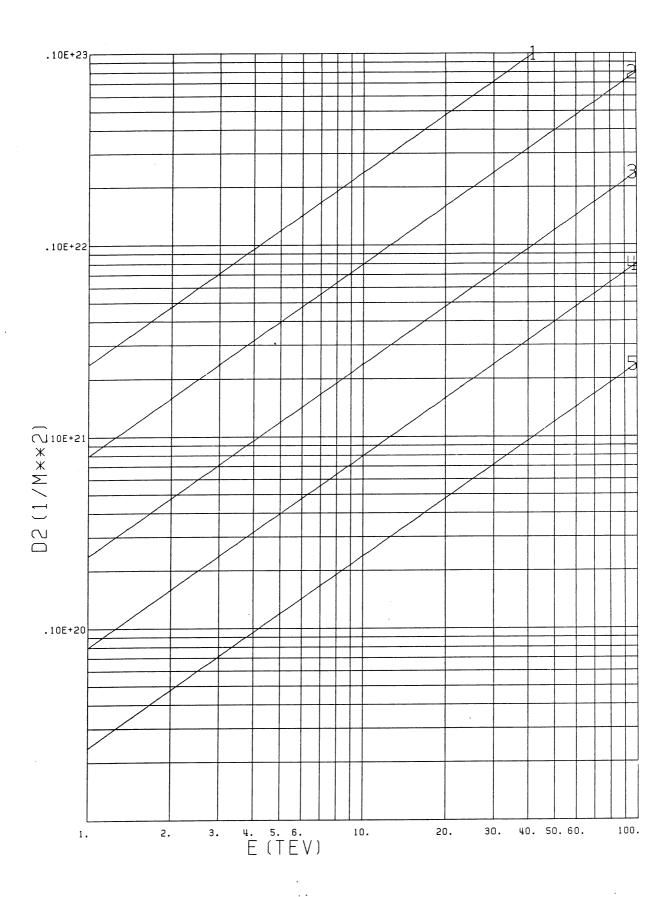
3. Phase space density  $D_2$  in  $m^{-2}$  versus beam energy E in TeV. The parameter is  $L\beta_t$ s, taking values  $10^{37}$ ,  $3.10^{37}$ ,  $10^{38}$ ,  $3.10^{38}$ ,  $10^{39}$ s<sup>-1</sup> for curves 1, 2, 3, 4, 5 respectively. For all curves  $\Delta Q = 0.003$ .
