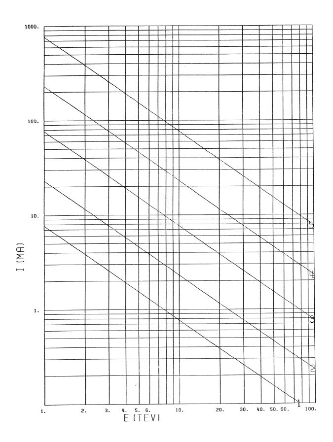
1. Circulating current I in mA versus beam energy E in TeV. The parameter is L $\beta_t$ , taking values  $10^{33}$ ,  $3.10^{33}$ ,  $10^{34}$ ,  $3.10^{34}$ ,  $10^{35}$  cm<sup>-1</sup>s<sup>-1</sup> for curves 1, 2, 3, 4, 5 respectively. For all curves  $\Delta Q = 0.003$ .
