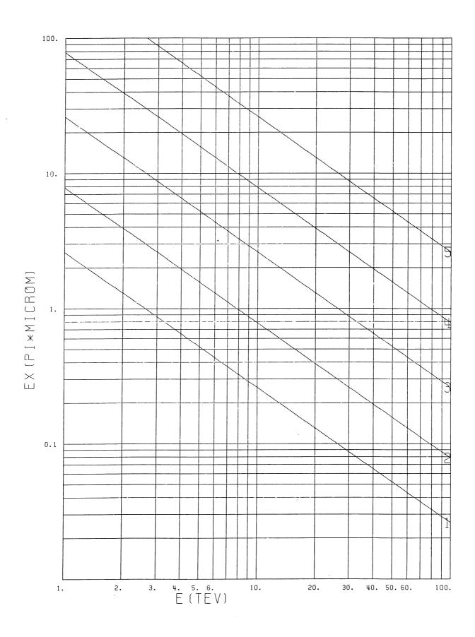
2. Beam emittance  $\varepsilon$  in  $\pi\mu$ m versus beam energy E in TeV. The parameter is L $\beta$ ts, taking values  $10^{37}$ ,  $3.10^{37}$ ,  $10^{38}$ ,  $3.10^{38}$ ,  $10^{39}$ s<sup>-1</sup> for curves 1, 2, 3, 4, 5 respectively. For all curves  $\Delta Q = 0.003$ .
