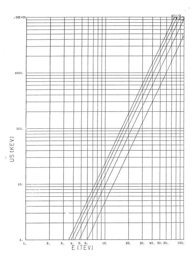
4. Synchrotron radiation loss  $U_S$  in keV versus beam energy E in TeV. The parameter is the dipole field B, taking values 2, 4, 6, 8, 10T for curves 1, 2, 3, 4, 5 respectively.
