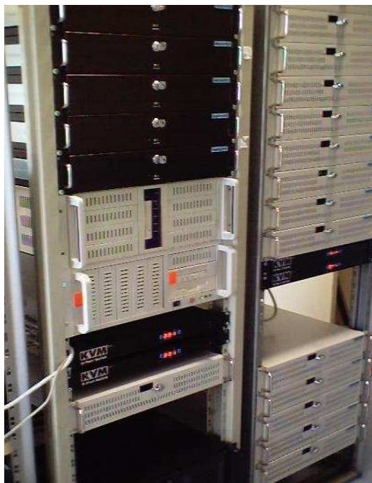
Figure 4.1: A visual impression of the cluster with the file server, a portal machine and the computing nodes
