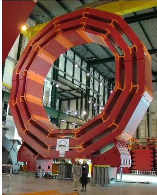
Figure 1.15: One of the five yoke rings. (Source: http://cmsinfo.cern.ch/outreach )
