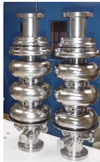
Figure 2: Both fabricated SRF-Gun cavities made from fine (left) and large grain material (right).
