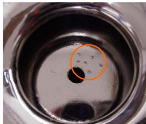
Figure 5: Photography of the defect pattern on endplate of the LG half-cell after re-treatment when defects appeared.
