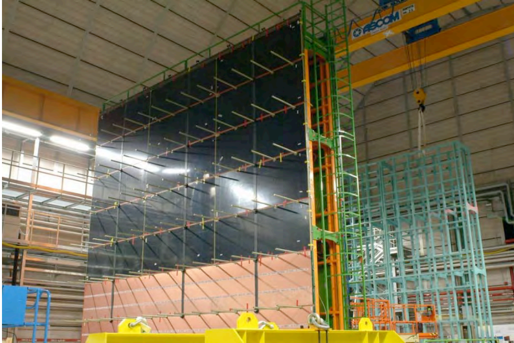
Figure 34. Detail of the assembly of the OPERA iron magnet.
