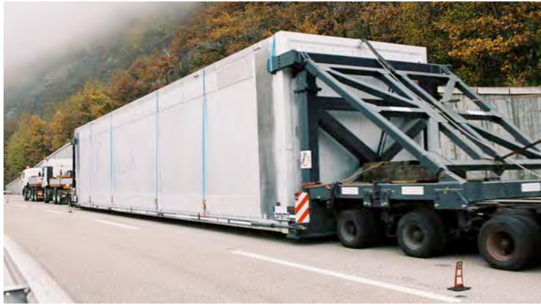
Figure 15: Picture taken during the transportation of a T600 half-module to LNGS. One of the two trolleys, attached to the aluminium vessels rear side, is well visible.
