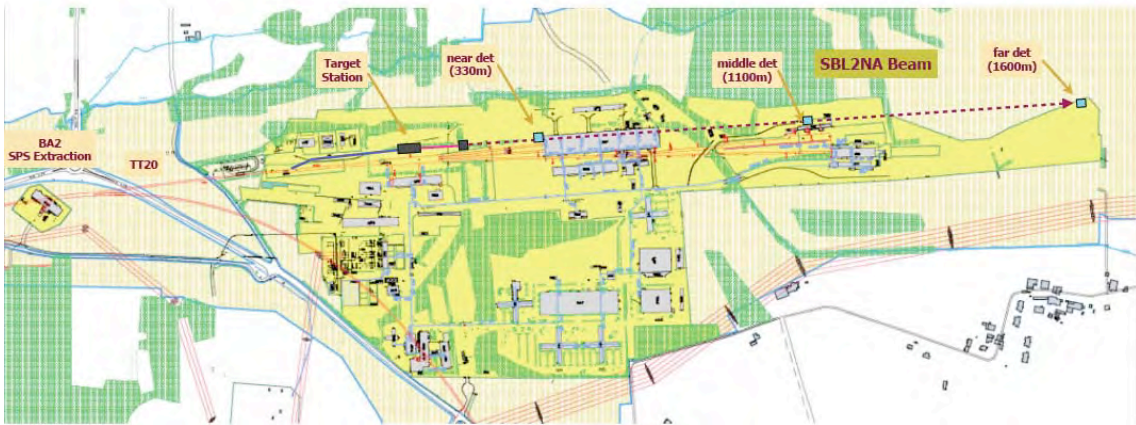
Figure 1. The new SPS North Area neutrino beam layout. Main parameters are: primary beam : 100 GeV; fast extracted from SPS; target station next to TCC2, ~11m underground; decay pipe: 100m, 3 m diameter; beam dump : 15m of Fe with graphite core, followed by muon stations; neutrino beam angle: pointing upwards; at -3m in the far detector ~5mrad slope. From I. Efthymiopoulos / CERN.
