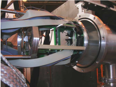
(c) The T-REX chamber installed at the target location. From [36].
