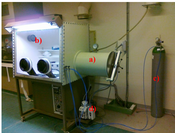
Figure II-7 – Gloves box used to do the material change to the target unit. In the picture: the pre-chamber (a), the gloves box main chamber (b), a bottle of Ar to fill both pre-chamber and main chamber (c) and a rotary pump (d).
