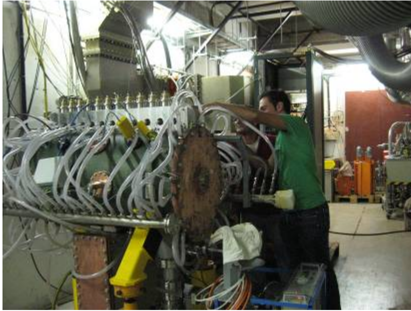
Figure 6 View of the high power installation of the DTL prototype in the SM18 bunker.
