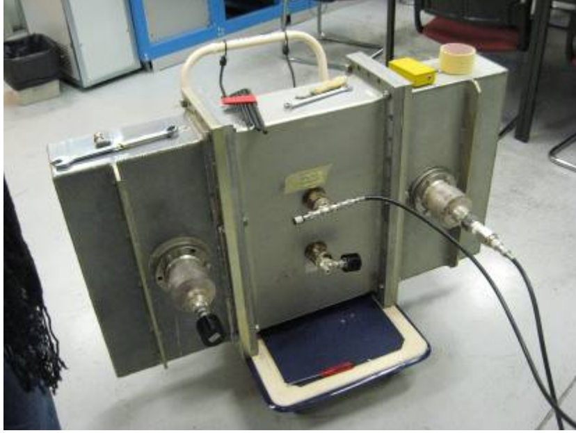
Figure 13 Directional coupler calibration.
