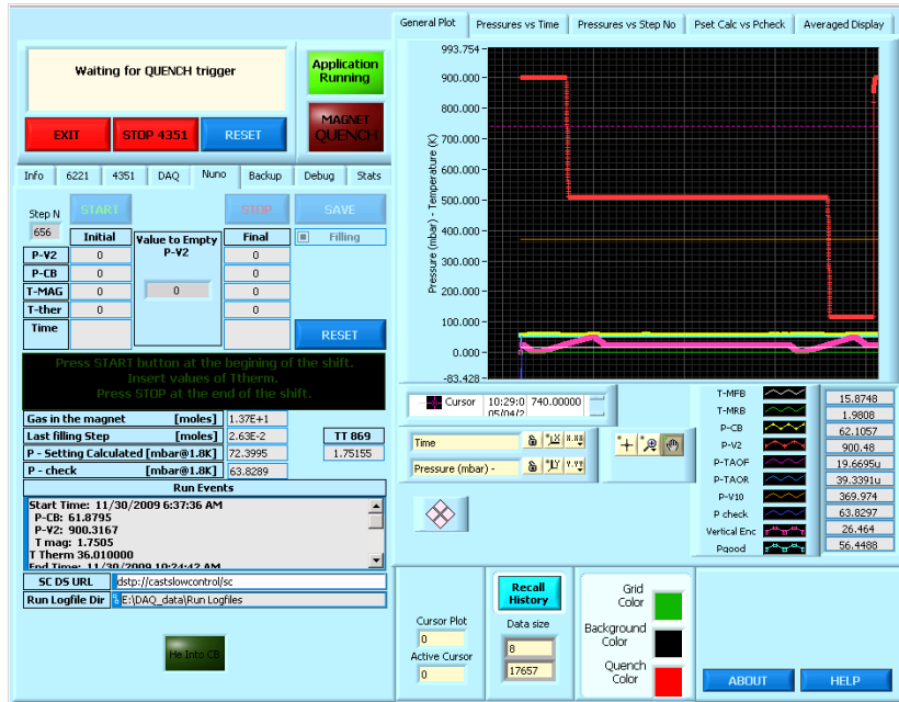
Figure 5-10: Display of the slow acquisition software. The left of the display contains different tabs for settings and controls. On the right side a histogram displays the evolution of the measured quantities.
