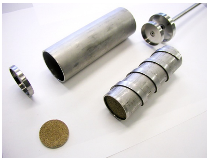
Figure 6-7: Exploded view of the construction of \text{LN}_2 charcoal trap
