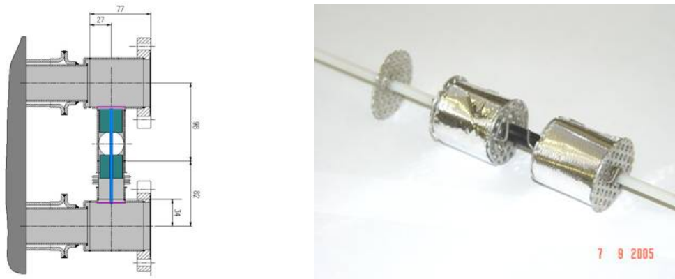
Figure 4-20: Left: Scheme with the position of the TAO dampers relative to the magnet face and the cold X-ray windows. Right: Photo of the TAO damper.
