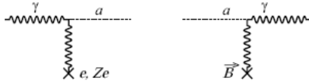
Figure 2-2: The Primakoff mechanism in the Sun (left) and the inverse process in a laboratory transverse magnetic field (right).
