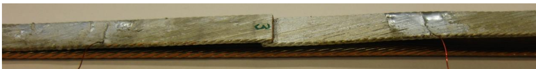
Figure 4: Sketch of FRESKA sample for four point resistance measurements at 4.3 K.
