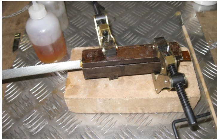
Figure 12: 120 mm resistively heated furnace for pre-tinning of the LHC busbar cable extremities.
