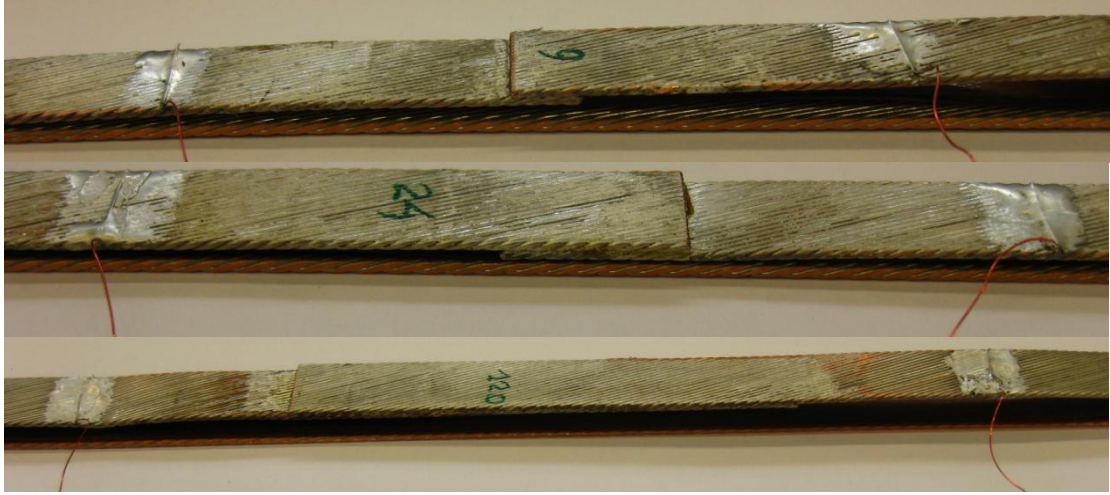
Figure 5: Photographs of the soldered cable splices with 3, 9, 24 and 120 mm intercable contact length.
