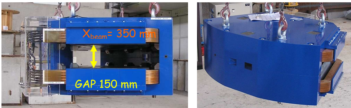
Figure 20. Bending Magnet for the 60 GHz bench.
