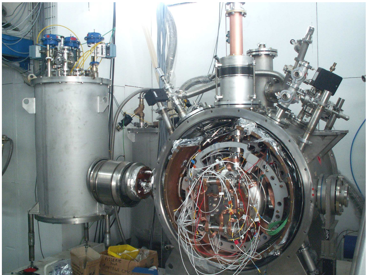
Fig. 6: Spoke Cryomodule and its cold box just before the cryogenic test.
