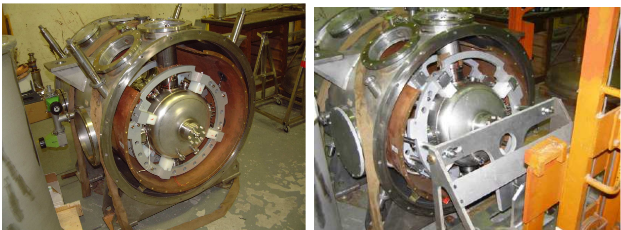
Fig. 2 Cryostat during assembly
