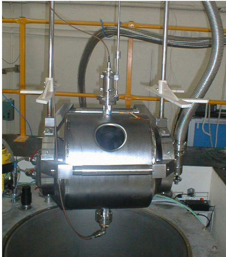
Fig 1 : Spoke cavity mounted on the vertical cryostat insert before testing
