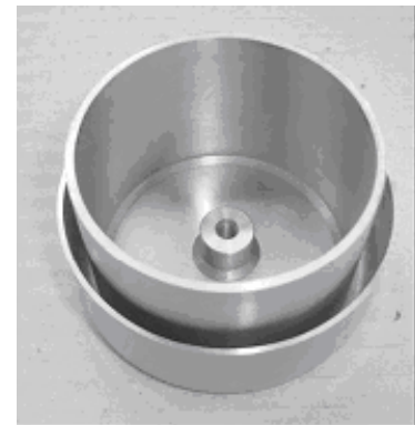
Figure 5.4. Detail of the tuning cup before welding to the resonator.
