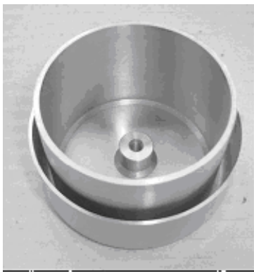
Figure 5.4. Detail of the tuning cup before welding.
