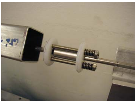
Figure 2: Fastening of two consecutive rods
