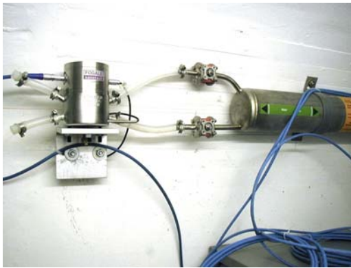
Figure 5: HLS sensor and hydraulic network
