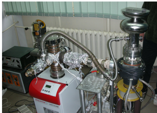
Figure 3: Setup for the plasma arc-deposition with the 1.6-cell cavity prepared for coating.
