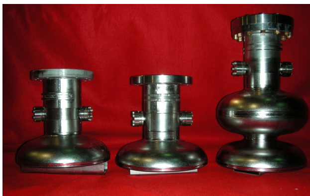
Figure 1: 1.3 GHz two half-cell and 1.6-cell SRF-gun cavities.
