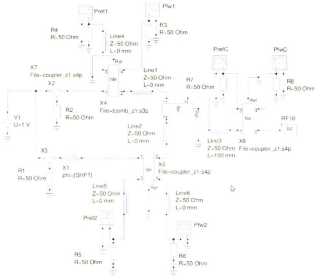
Fig. 9. The QUCS model of the RF-Gun control system.
