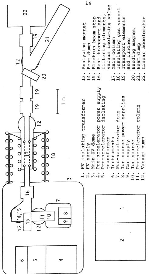
Conceptual layout of a spallation breeder dc injector. Figure 1.
